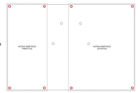
Place your throttle and joystick on the main plate and drive 8 Allen screws (M5x16) with 8 (M5) cups to fix it firmly.
