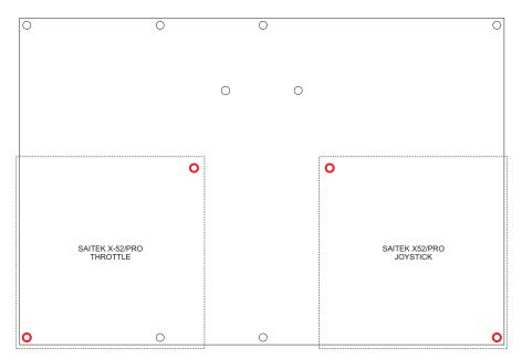
Place your SAITEK X52/PRO throttle and joystick on the main plate and drive 4 conical screws (M4x55) with 4 washers(4) and 4 (M4) cups to fix it firmly.
