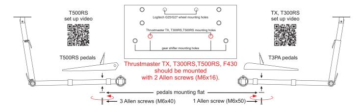
Place your pedals in the centre of the stand and drive 3 Allen screws (M6x40) to fix it firmly. Thrustmaster T3PA pedals should be mounted with 1 Allen screw (M6x50). Allen screw (M6x50) is for G27 and T3PA pedals only.
