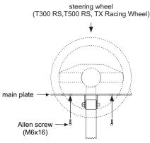
Drive 2 M6x16 Allen screws to connect the steering wheel (T300RS, T500 RS and TX Racing Wheel) with the main plate (without shifter plate - see set up video).
