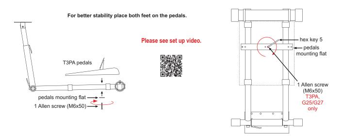
Place your T3PA pedals in the centre of the stand and drive 1 Allen screws (M6x50) to fix it firmly. Allen screw (M6x50) is for G27 and T3PA pedals only.
