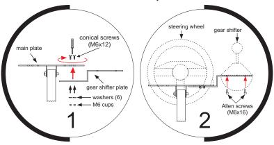
Put your wheel on the main plate and drive two Allen screws (M6x16) to fix it firmly. Drive another two screws (M6x16) to fix the gear shifter to the gear shifter plate.
