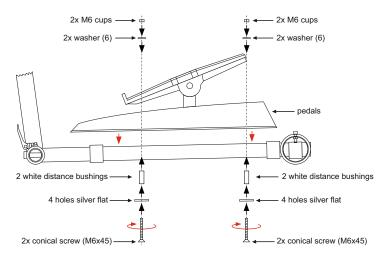
Place your pedals on the base of the stand and drive 4 conical screws - gradually (M6x45) with 4 white distance bushings from the bottom to 4 hole silver flat.
