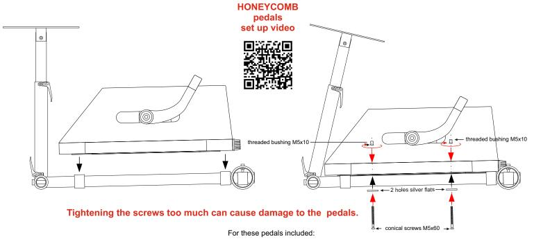
4 conical screws (M5x60), 4 threaded bushings (M5x10), 2 silver pedal flats
