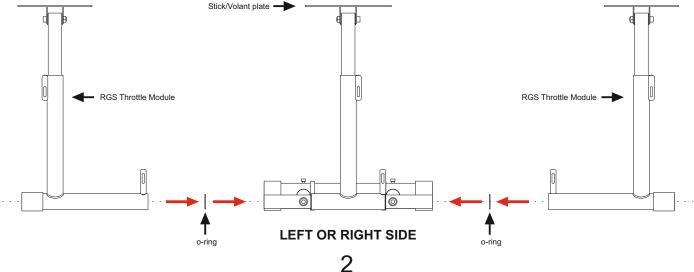
Secondly attach the Volant and Throttle to the Wheel Stand Pro stand. Please scan QR code to watch set up video
