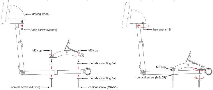
Place your pedals on the stand and drive 4x conical screws M6x55, 4x M6 cups and fix it firmly with 4x pedals flat plates.
